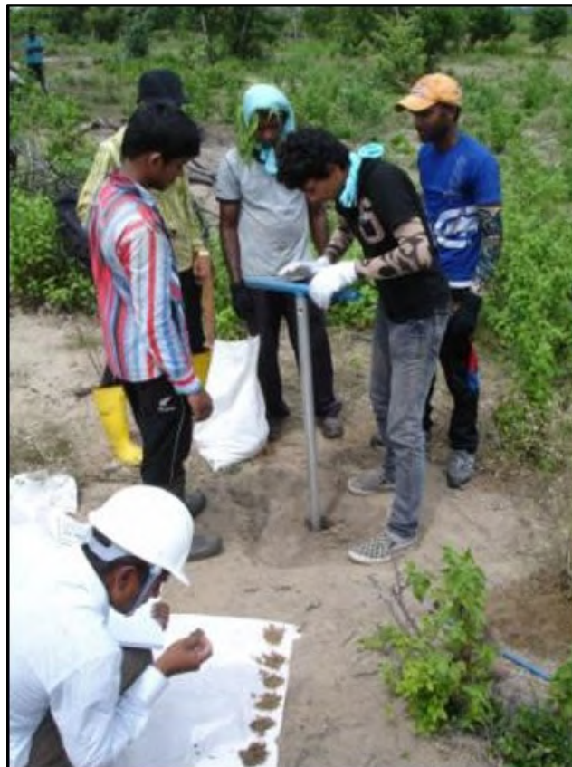
Figure 3.9 Auger drilling and logging in EMP North
